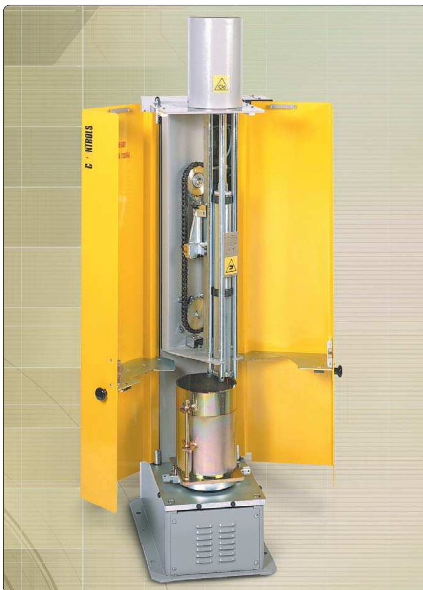
33-T8500 Series with CBR mould. View with open doors. Closing the doors all moving parts are shielded and micro switches prevent operation with the doors open. This design makes maintenance extremely easy. The upper frame housing the rammer mechanism moves automatically angularly for the total surface compaction of the 152.4 mm dia. (6") moulded specimens. The rammer pick-up has a cam system for accurate height release and is made of highly resistant material for trouble free long life. The rammer portion is moved across the sample surface by a cogged gear whilst the mould rotates on the lower table.
