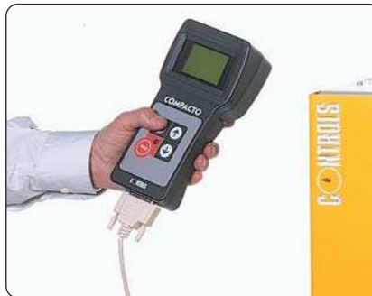
33-T8532. Detail of the hand held control panel. The user-friendly software is set out in an easy to follow logical sequence through each stage of the compaction. The end of each compaction stage is indicated by a visual and acoustic signal.
