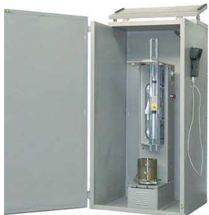
Automatic compactor fitted in noise reduction cabinet.
