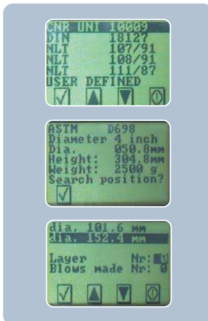
33-T8532. Detail of the large 240x128 pixel display. The displayed information can be pre-set in English, French, German, Spanish and Italian. The above are just some of various possibilities that the system offers.
