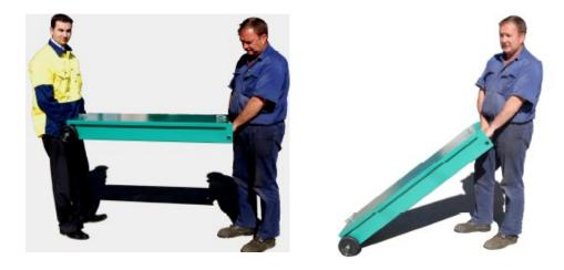
The container can be carried by two people or wheeled by one person. Total mass of container and DCP equipment is  $\pm$  55kg.
