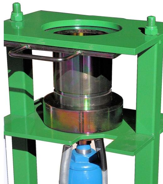
Extruder set up for Compaction Mould extrusion
