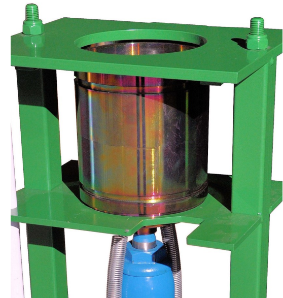
Extruder set up for CBR Mould extrusion
