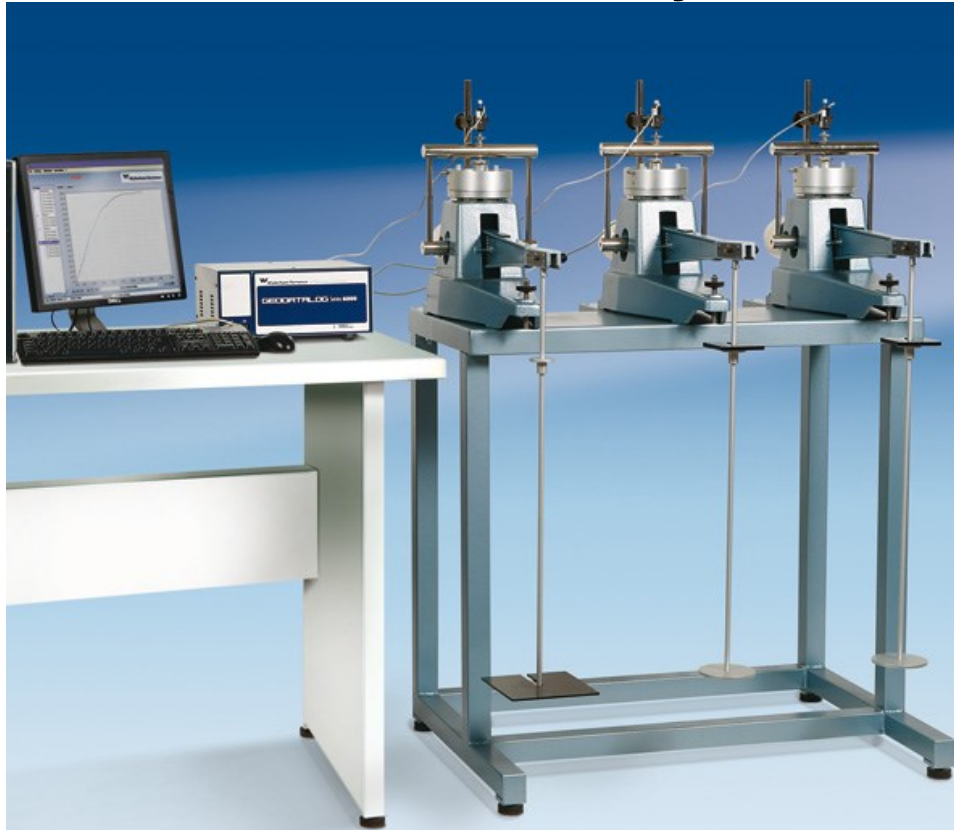
26-WF0338/A Permeability at- tachment fitted to the 26- WF0302 with 26- WF0320 cell
