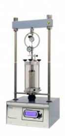
Standard triaxial system with analogue measurement
