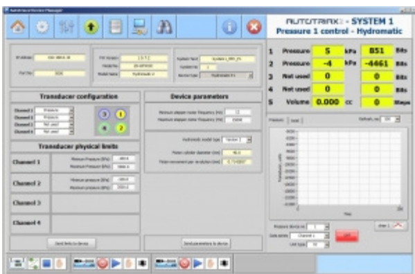
Device Settings panel for Hydromatic 2 pressure/volume data acquisition and control device showing settings for the four channels
