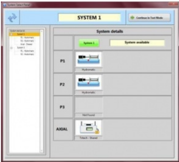
System Selection panel showing two triaxial systems are available, with one shared Tritex compression frame
