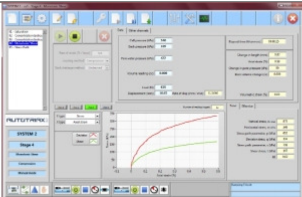
Deviator and shear stress plotted against axial strain during a monotonic shear stage
