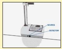
Moisture content is measured in a nondestructive test mode. Moisture is determined through the detection of thermalized neutrons ("fast" neutrons which have been slowed by the hydrogen present in the material, normally in the form of water).
