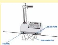
The backscatter mode is a rapid and nondestructive means of testing materials that are approximately 4 in. (10 cm) in depth. The gamma source remains inside the gauge and the gamma rays that are scattered back toward the detectors are counted, determining the density count for the material. This mode of testing is usually used on asphalt and concrete.
