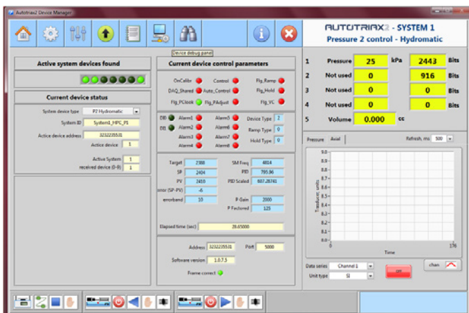
Debugging panel of Autotriax 2 software for automatic triaxial tests
