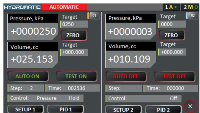
Auto Control (screenshot): Automatic execution of pre-programmed steps of pressure and/or volume change.
