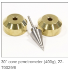
30° cone penetrometer (400g), 22-T0029/8
