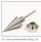
30° cone penetrometer (100g), 22-T0029/7
