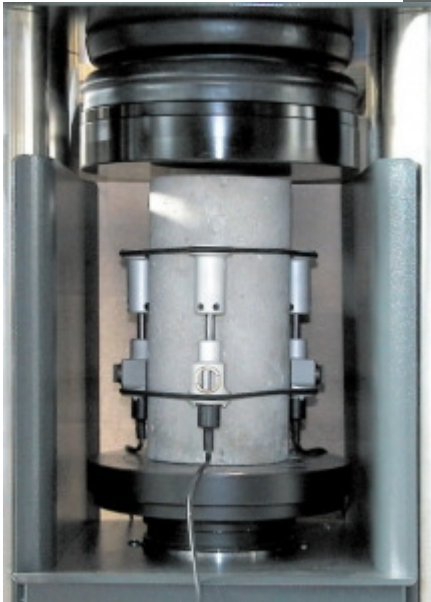
Specimen fitted with 55-C0222/F compressometers
