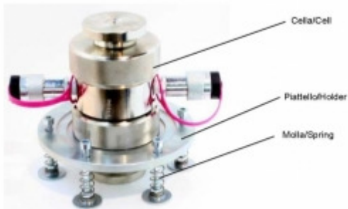
Hoek cell 45-D0556 supported by holding device model 45-D0556/H
