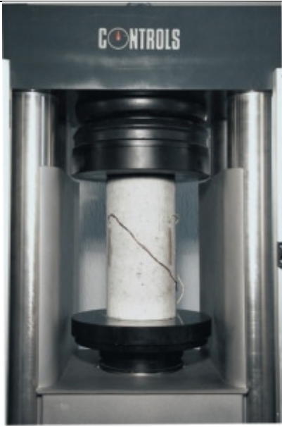
Determination of Elastic Modulus using surface-mounted strain gauges
