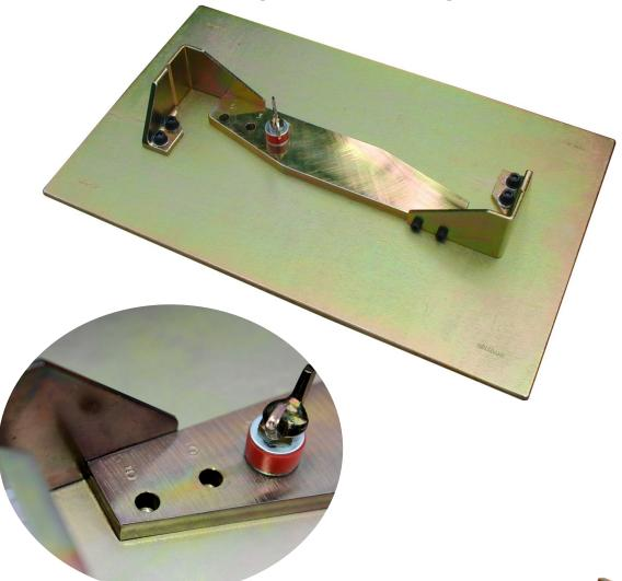
The Proportional Caliper is used to determine the proportion of flat particles, elongated particles and flat elongated particles found in those fractions of a coarse aggregate retained on a 9.5mm Test Sieve.
