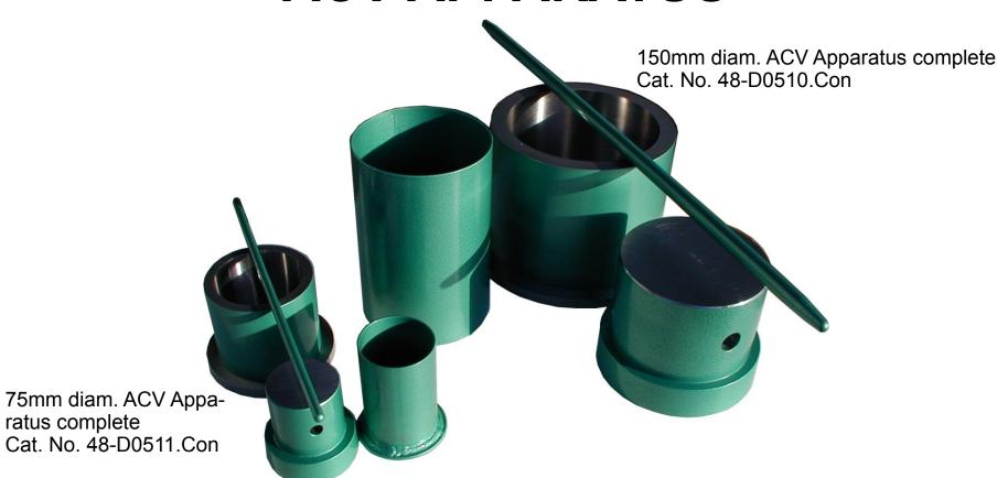
ACV Apparatus (75 & 150mm Diameter)
