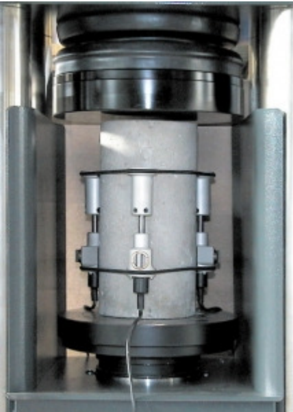
Specimen fitted with 55-C0222/F compressometers
