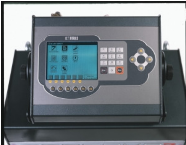
Detail of MCC display used basically for calibration purpose
