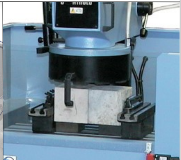
Grinding Machine with standard cube Clamping device
