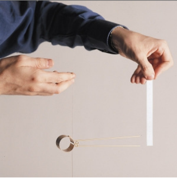
Use of the extensibility of mould apparatus 62-L0025/4
