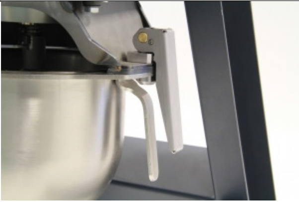
65-L0512 - Detail of the quick bowl mounting device
