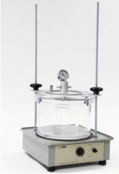
De-airing agitation device including vacuum pyknometer 75-D1122 and electro-magnetic vibro-
