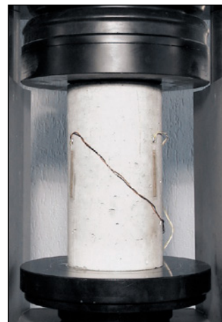
Specimen fitted with 55-C0222/F compressometers
