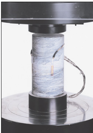
Determination of Elastic Modulus using surface-mounted strain gauges
