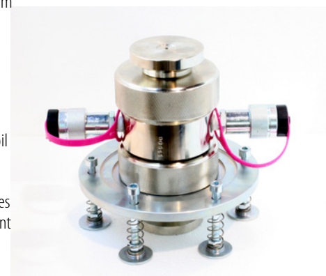
Hoek cell 45-D0566 supported by holding device model 45-D0556/H
