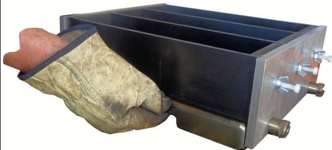
Lifting the Mould without Handle or Lifting Device
