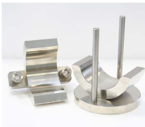
Marshall stability mould for 4" dia.
