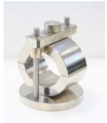
Marshall stability mould for 4" dia. specimens 76-B0033
