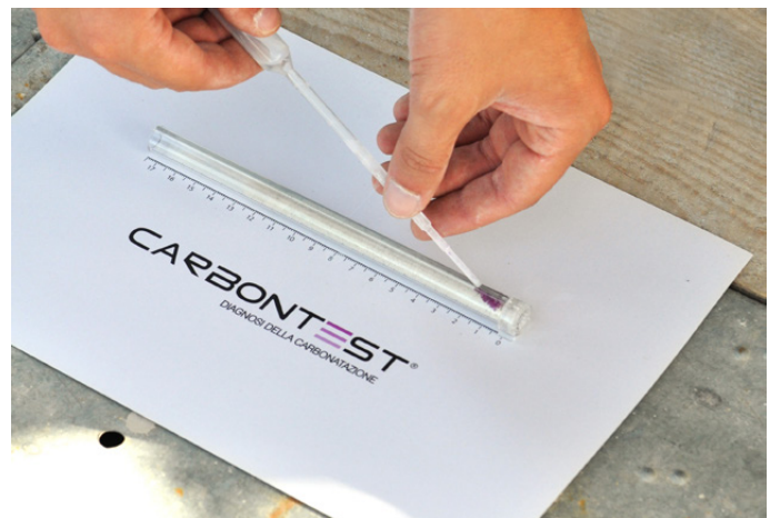
Application of phenolphthalein solution on the test tube with concrete powder
