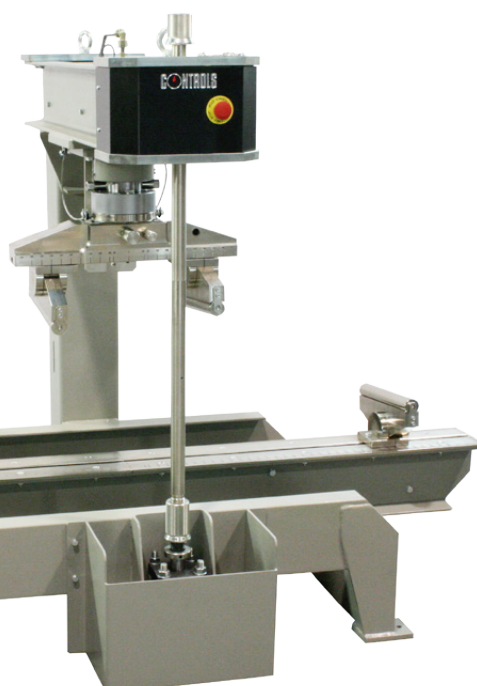
300 kN UNIFLEX frame (50-C1601/FR) fitted with accessories for flags testing (50-C1601/2 and 50-C1601/KIT)
