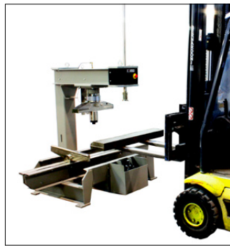
Easy specimen loading with forklift
