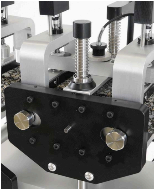
Detail of Servo-pneumatic Four Point Bend Apparatus
