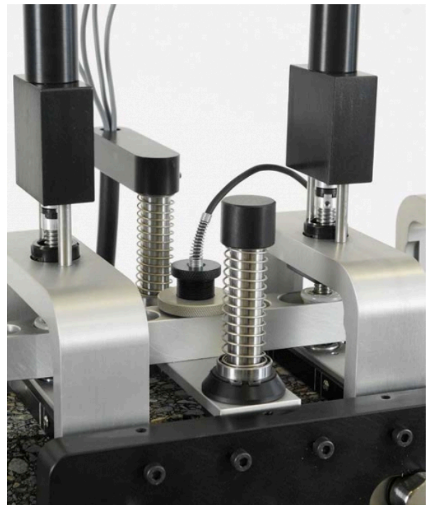
Detail of Servo-pneumatic Four Point Bend Apparatus
