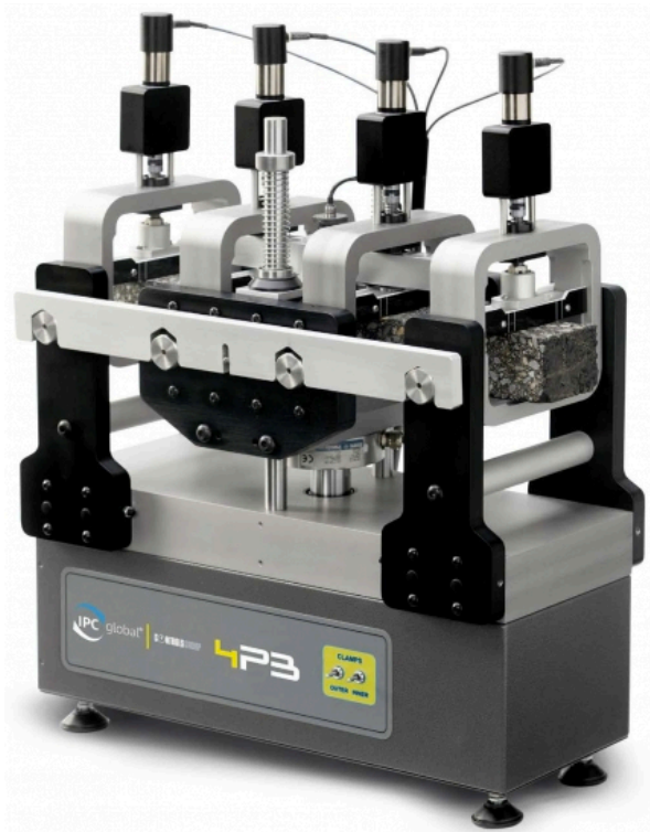
Servo-pneumatic Four Point Bend Apparatus
