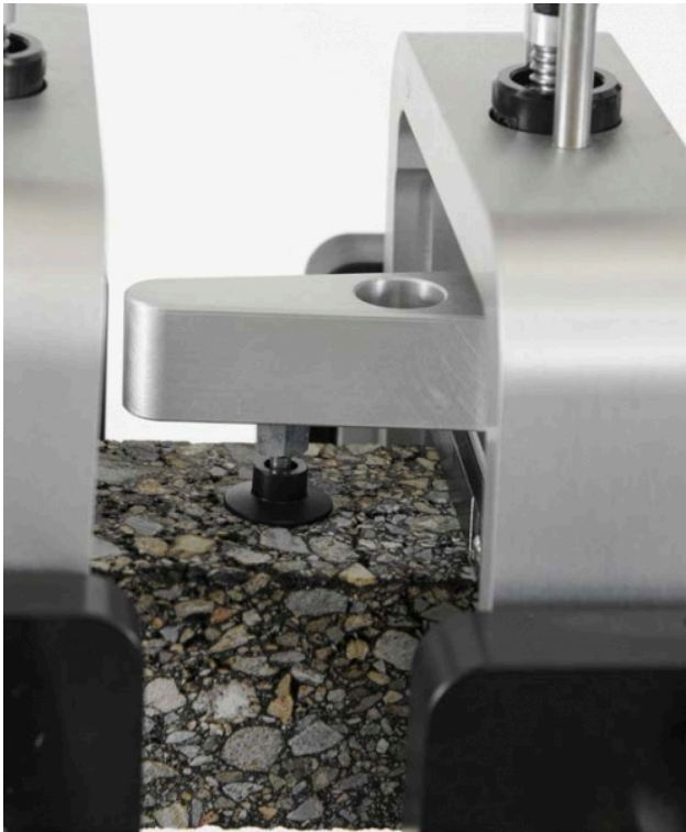
Detail of Servo-pneumatic Four Point Bend Apparatus
