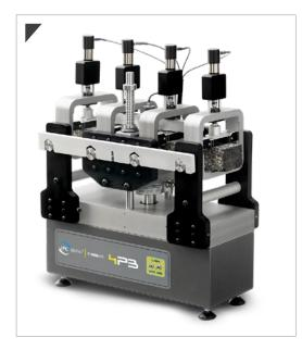
The Servo-Pneumatic Four Point Bend Apparatus comprises of a pneumatically powered loading system, a beam cradle, an optional environmental chamber, IMACS Integrated Multi-Axis Control System and UTS test application software.
