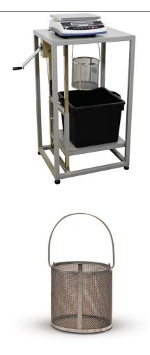
Specific gravity frame with electronic balance and basket
