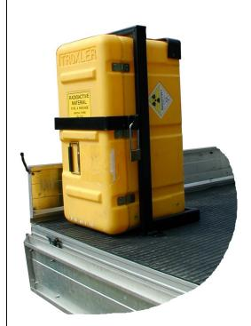
The frame is secured to the tray with bolts and the gauge in its case is inserted in an upright position. The gauge is accessed by simply lowering the vehicle tailgate, unlocking the frame and opening the case. The gauge slides straight out. No more lifting of the gauge up and over the sides of the vehicle.
