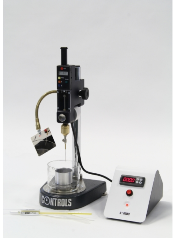
Digital electronic semi-automatic penetrometer complete with micrometer vertical adjustment and adjustable electronic timer of the fall time
