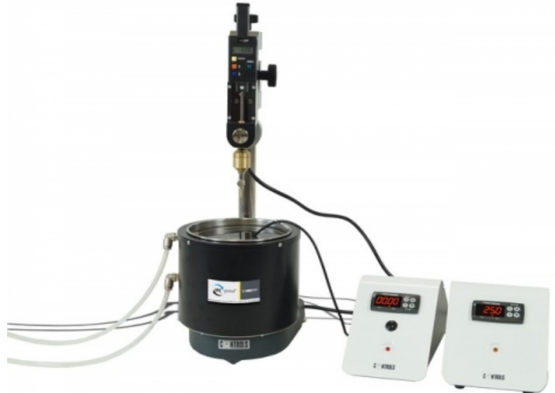
81-B0101/E Digital electronic semi-automatic penetrometer and 81-PV0102 digital water bath with thermoregulatory and immersion temperature probe
