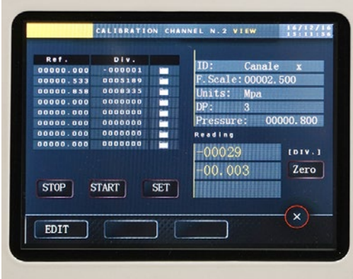
Pressure transducer calibration menu.
