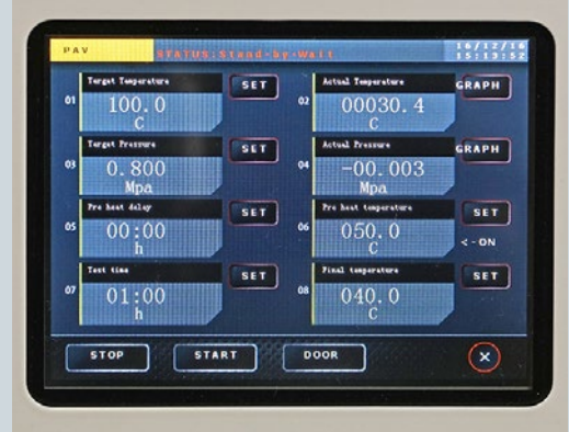
Temperature and pressure target values vs actual values.
