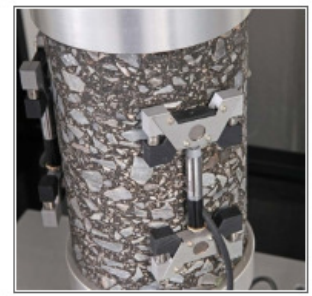
Dynamic Modulus Test for AST Pro and AsphaltQube 79-PV72500
