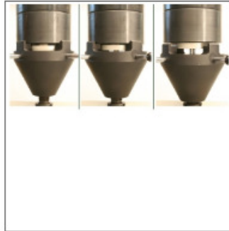
No Load Pre Load (25 N) Load (525 N) Detail of the weight positioning system, allowing to pass from No-Load to Pre-Load phase, then to Poad phase in a very fast, precise and safe way: by rotating the lower part, the load conditions are
