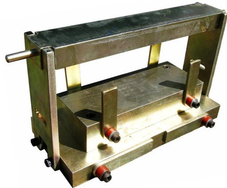
Brazil Jig with Adaptor set up for 100 mm Cylinder Cat. No. 50-C9010/A.Con
