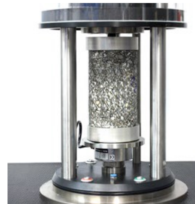
Stress Sweep Rutting (SSR)
