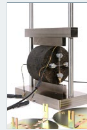
AASHTO T322/TP9, ASTM D7369, & NCHRP 1-28A APPENDIX 1
