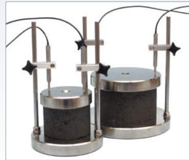
Permanent Deformation Creep Test
