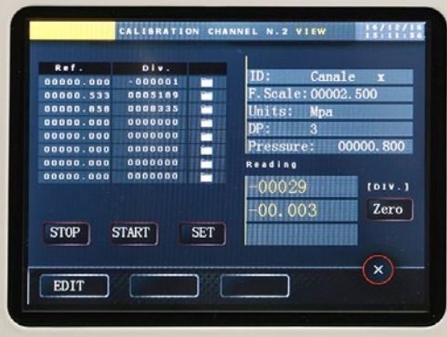
Pressure transducer calibration menu.
