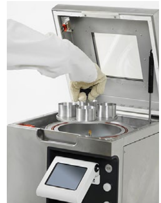
Double face sample rack positioning
