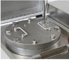
Detail of certified pressure vessel and cover locking switch
