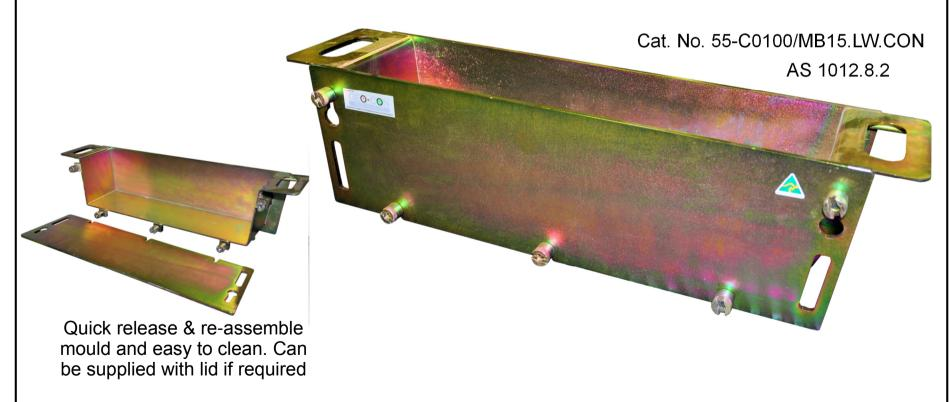
Lightweight 150 x 150 x 510 Flexure Beam Mould
