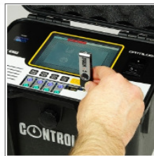
Data acquisition unit DATALOG 8 model 82-P9008/F - Detail of removable USB pen drive
