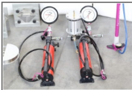
32-D0548/D: Detail of hydraulic pumps fitted with Bourdon gauges and pressure transducers
