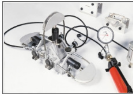
32-D0548/A: Detail of the shear box apparatus fitted with 5 digital gauges (4 vertical and 1 horizontal)
