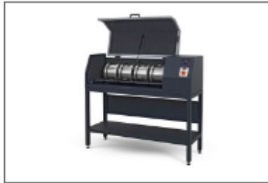
Micro-Deval testing machine model 48-D5242/A with base accessory 48-D5242/A1 and testing drums
