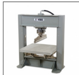
Flexure testing on concrete flagstones with 200kN high stiffness frame 50-C1511/FR.
