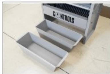
Large capacity sample splitter model 15-D0430/A
