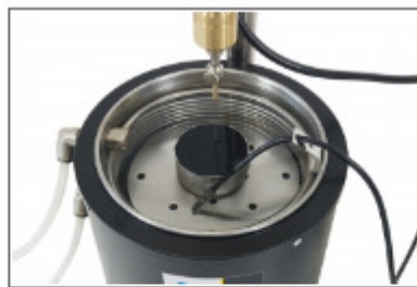
Detail of PT100 immersion probe
