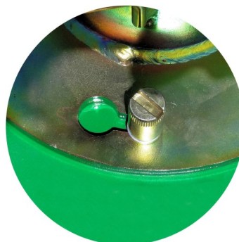
Quick coupling and release system for mounting the Moulds on to the Table
