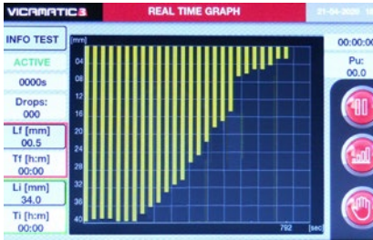
Setting time plot shown in real time on VICAMATIC-3 display
