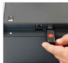
Communication ports are positioned on the rear side. LAN port is suitable for connection to PC or to LAN-hub, that creates a network with up to 32 independent units controlled by a single PC. USB port is used for data download to PC and firmware upgrade.
