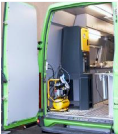
Gyrocomp installed in a van as a road mobile laboratory
