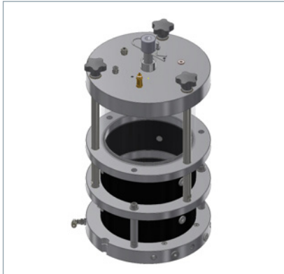
Triaxial Cell – 150 and 100mm specimens
