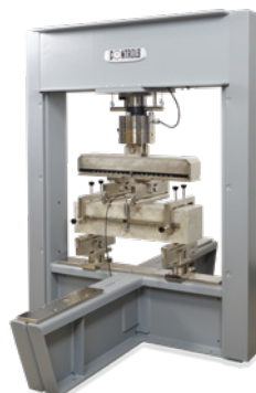
Deflection test on Steel Fiber Reinforced Concrete beams to EN 14651 [CMOD Method] and to UNI 11039 (CTOD method)
