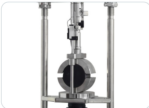
Set for performing MARSHALL test (accessories have to be ordered separately).
